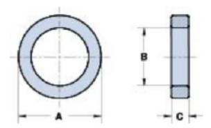
OD(A) = 0.375 in / 9.5 mm +/- 0.25 mm ID(B) = 0.187 in. / 4.75 mm +/- 0.10 mmHt(C) = 0.125 in. / 3.3 mm +/- 0.25 mm
